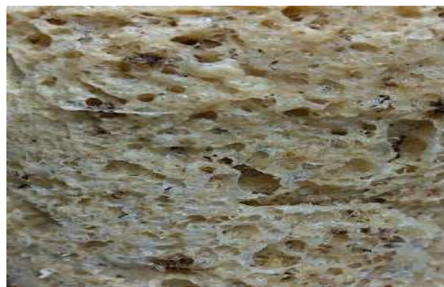
Figure 2b. Structure of foam developed using PEG: JSDL-90:10
