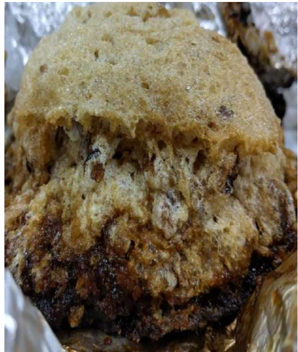
Figure 3d. Foam developed using PEG: JSDL-60:40
