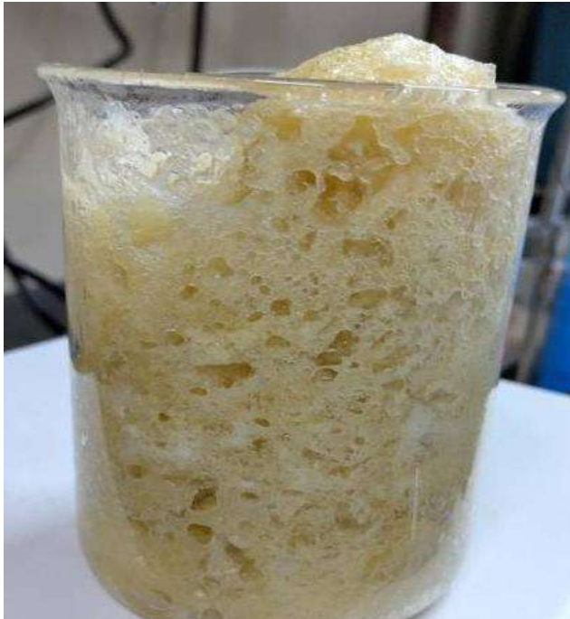
Figure 3a. Foam developed using PEG: JSDL-100:0
