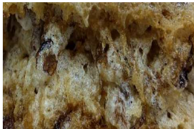
Figure 2d. Structure of foam developed using PEG: JSDL-60:40
