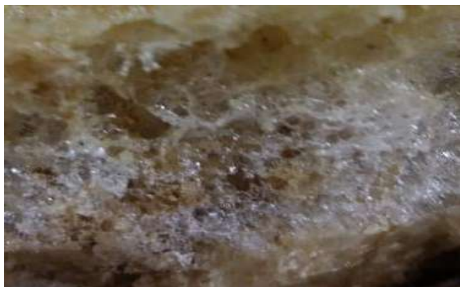
Figure 2c. Structure of foam developed using PEG: JSDL-80:20
