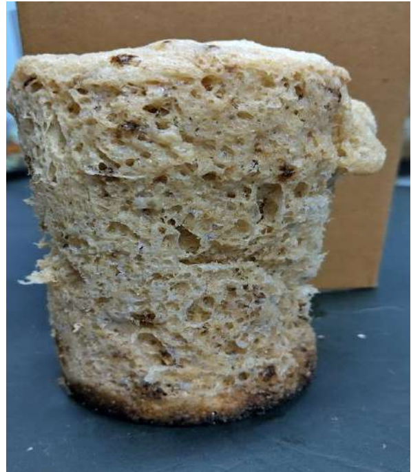
Figure 3b. Foam developed using PEG: JSDL-90 :10
